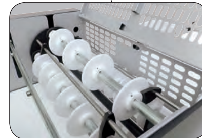
Longitudinal cutting disks and Transversal cut guillotine
