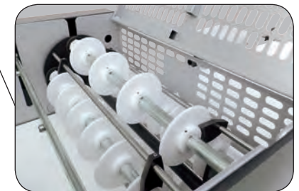
Longitudinal cutting disks and transversal cut guillotine.
